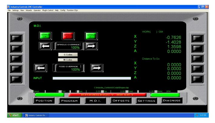
The MDI page (Manual Data Input) is used for a single movement or to execute a series of codes for testing or what ever short program you may want to do.
