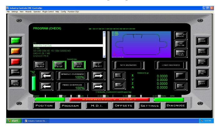
This page is where programs are loaded in to memory and the actual program is executed from. Functions on this screen are Edit, Tool path Graphics, Single block, Optional stop, Z axis inhibit, Spindle and Feed rate overrides, Cycle start, Feed hold and Reset. Conversational functions are available from here as well along with the "distance to go" position.
