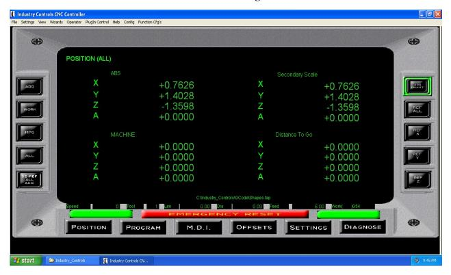
This page displays Machine Position, Absolute Coordinate Position, Encoder reading and distance to go. The left side of the screen has the ability to select and display only one of the positions at a time.
