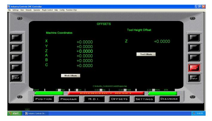
Offsets are used to establish a new zero position for programming a part. There are 2 basic types of offsets. They are work coordinates and height offsets.
