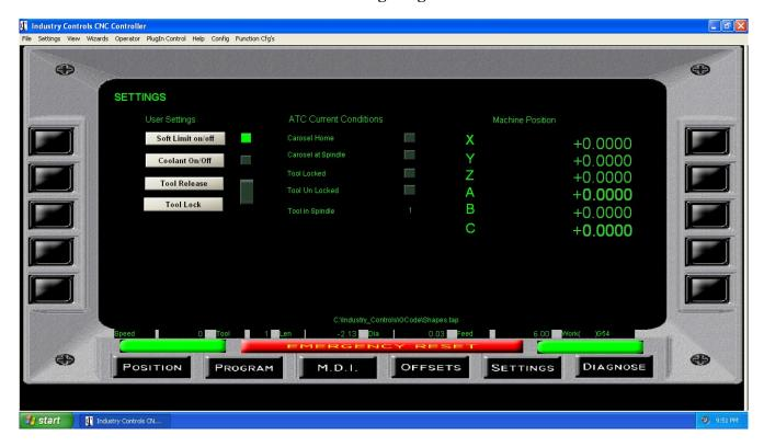
The settings page is used for numerous things. As shown on this configuration the soft limits are turned on. This is a stored value how much travel you have. If your program will exceed the allowable limits, you will get a warning prior to running the program. It also displays an automatic tool changer current positions or anything special or frequently viewed that you might find necessary. It also displays all 6 machine coordinate locations.
