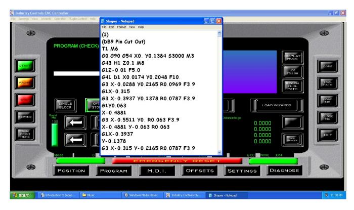
By pressing the Edit button, the "G" code editor will open in notepad or any specified text editing software you have installed on the PC. This makes using software's such as Bobcad, Mastercam or what ever you choose very easy.
