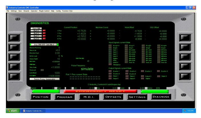
This page displays all current conditions of Inputs and Outputs. It is the simplest way to troubleshoot. It makes repairs fast and easy to find as it tells you exactly what the Control sees.
